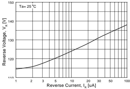
**Figure 1. Reverse Voltage vs Reverse Current**
