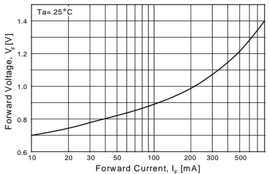
**Figure 5. Forward Voltage vs Forward Current**
