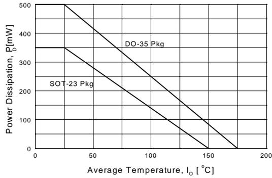
**Figure 9. Power Derating Curve**
