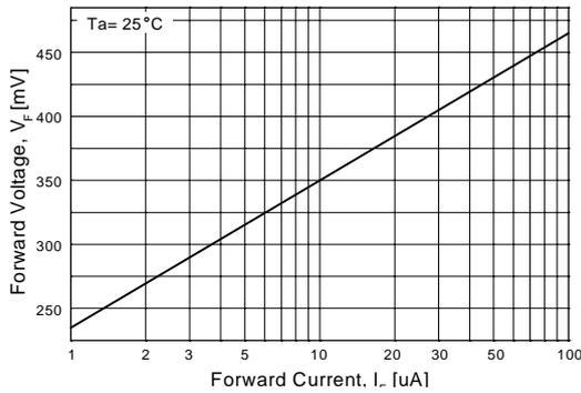
**Figure 3. Forward Voltage vs Forward Current**
