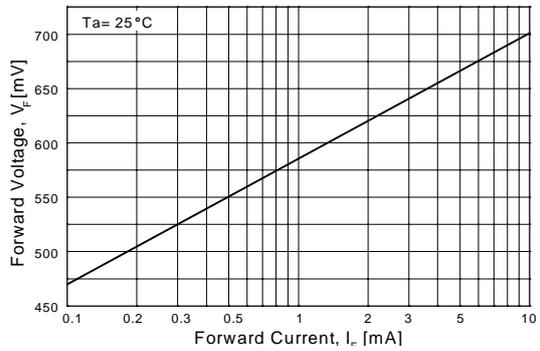
**Figure 4. Forward Voltage vs Forward Current**
