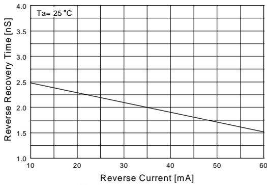
**Figure 7. Reverse Recovery Time vs Reverse Current**
