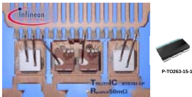
Fig. 10: Smart semiconductor full-bridge with full protection and diagnostics, realized in chip-by-chip technology
