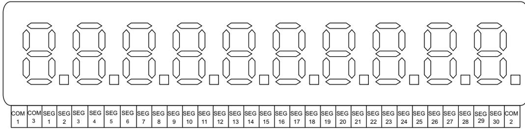
LCD driving system 1/2 bias, 1/3 duty, 3V
