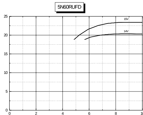
Figure 3.4.1 The Relationship between V_{GE} and the Maximum Current that can flow in the IGBT (5N60RUFD)
