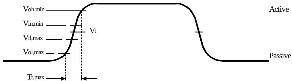
Figure 9. SAE J1850 VPW Waveform
