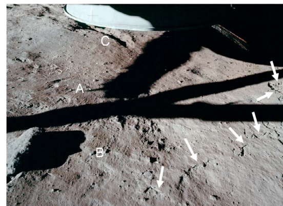
Figure 9. Apollo 11 surface. Arrows show the contact between the upper soil layer and the sublayer. Area A has numerous radial erosional remnants, each headed by gravel. Area B has a set of short longitudinal features in the form of downward steps from the impingement point. Trench C was caused by the soil contact probe during landing. The engine nozzle is visible at the top. (Detail from NASA photograph AS11-40-5921HR.)
