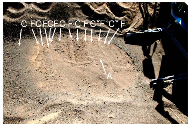
Figure 21. Lamination in soil exposed during case 7 (contrast enhanced). F, fine layers; C, coarse layers; C*, presumed location of coarse layers completely removed by plume; A, unheaded erosional remnants. Note brightness in eroded region, in this case due to removal of coarse particles.
