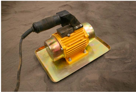
Figure 13. Vibrational hand compactor used to densify the tephra.
