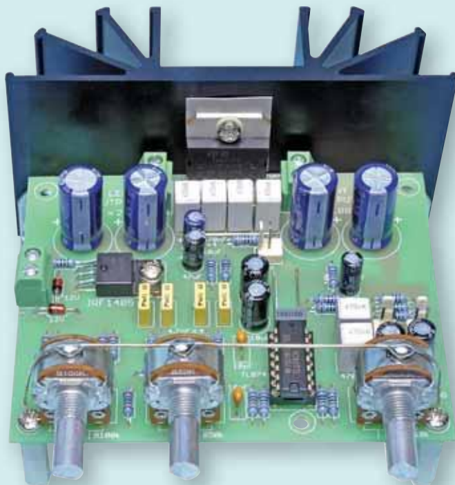
Fig.4: follow this layout diagram to build the PC board. Make sure that all polarised parts are correctly oriented and don't get the pots mixed up.
