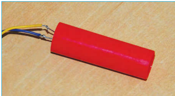
Fig.6. A coloured cap from a marker pen can be used over the LED to give a more diffused glow
