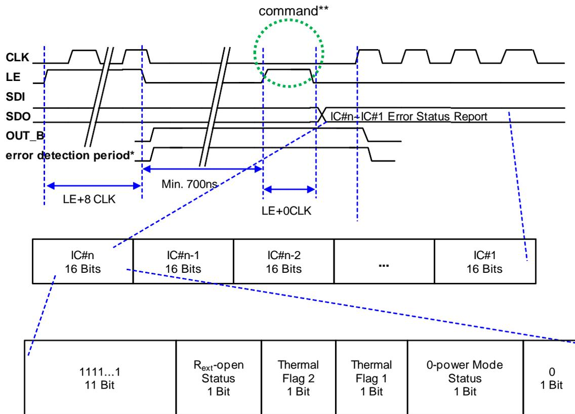
\*For the correctness of the error message, MBI5038 releases the error detection period only when receiving one LE pulse containing 0 CLK and CLK is active. During the error detection period, MBI5038 will force OUT\_B off and perform the compulsory error detection. MBI5038 releases the error detection period when LE falling (any commands).
