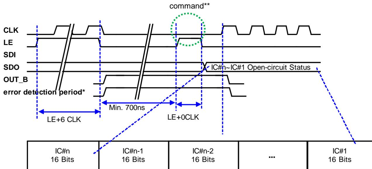
\*For the correctness of the error message, MBI5038 releases the error detection period only when receiving one LE pulse containing 0 CLK and CLK is active. During the error detection period, MBI5038 will force OUT\_B off and perform the compulsory error detection. MBI5038 releases the error detection period when LE falling (any commands).
