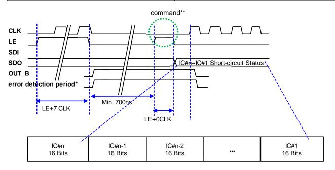
\*For the correctness of the error message, MBI5038 releases the error detection period only when receiving one LE pulse containing 0 CLK and CLK is active. During the error detection period, MBI5038 will force OUT\_B off and perform the compulsory error detection. MBI5038 releases the error detection period when LE falling (any commands).
