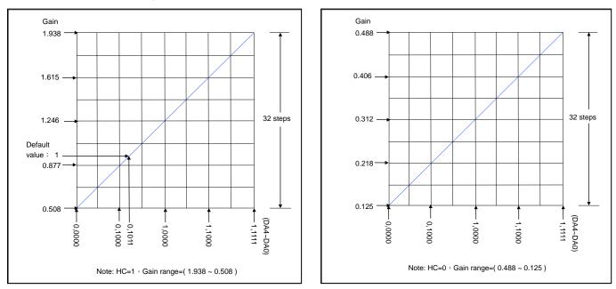
The bit 5 to bit 0 of the configuration register set the gain of output current, i.e., G. As totally 6-bit in number, i.e., ranged from 6'b000000 to 6'b111111, these bits allow the user to set the output current gain up to 64 levels.
