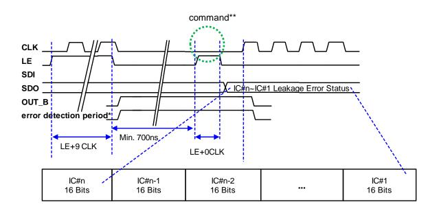
\*For the correctness of the error message, MBI5038 releases the error detection period only when receiving one LE pulse containing 0 CLK and CLK is active. During the error detection period, MBI5038 will force OUT\_B off and perform the compulsory error detection. MBI5038 releases the error detection period when LE falling (any commands).
