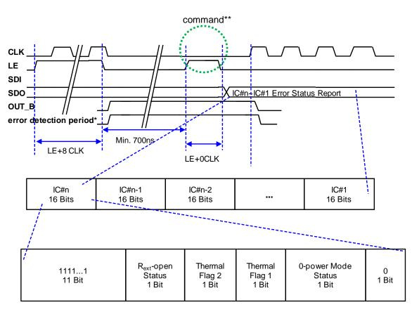
\*For the correctness of the error message, MBI5038 releases the error detection period only when receiving one LE pulse containing 0 CLK and CLK is active. During the error detection period, MBI5038 will force OUT\_B off and perform the compulsory error detection. MBI5038 releases the error detection period when LE falling (any commands).
