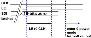
Until the PWM gray scale data are all none zero and must wait 1 min-second, the output will be turn on and automatically leave the 0-Power mode.
