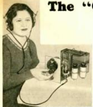
The 1-Tube "Oscillodyne" in actual operation. This is the set shown on our front cover.
