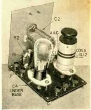
Rear view of the "Oscillodyne" with parts labeled to correspond with those in the diagram.
