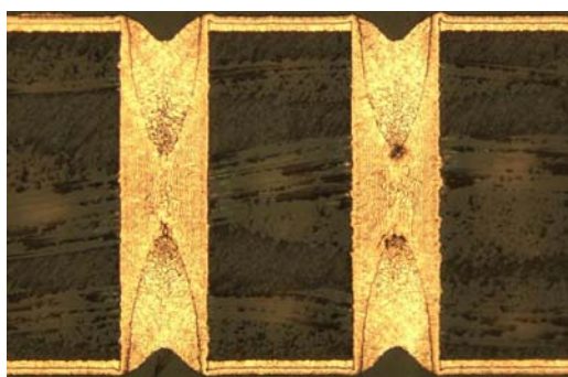
Fig 15: Copper filled 400µm core with 100µm diameter holes showing small voids.
