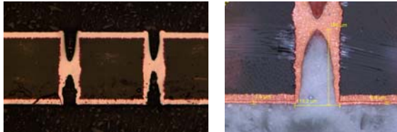
Fig 7: 400 \mu\text{m} thick core with 100 \mu\text{m} TH plated within 15 min. Right detail showing 9 \mu\text{m} plated Cu on the surface while > 50 \mu\text{m} Cu plated in the middle of the via
