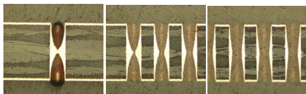
Fig. 5: Difference between isolated and clustered through holes. Left: isolated, right clustered TH with 200 µm pitch, middle through holes at the edge of such a cluster
