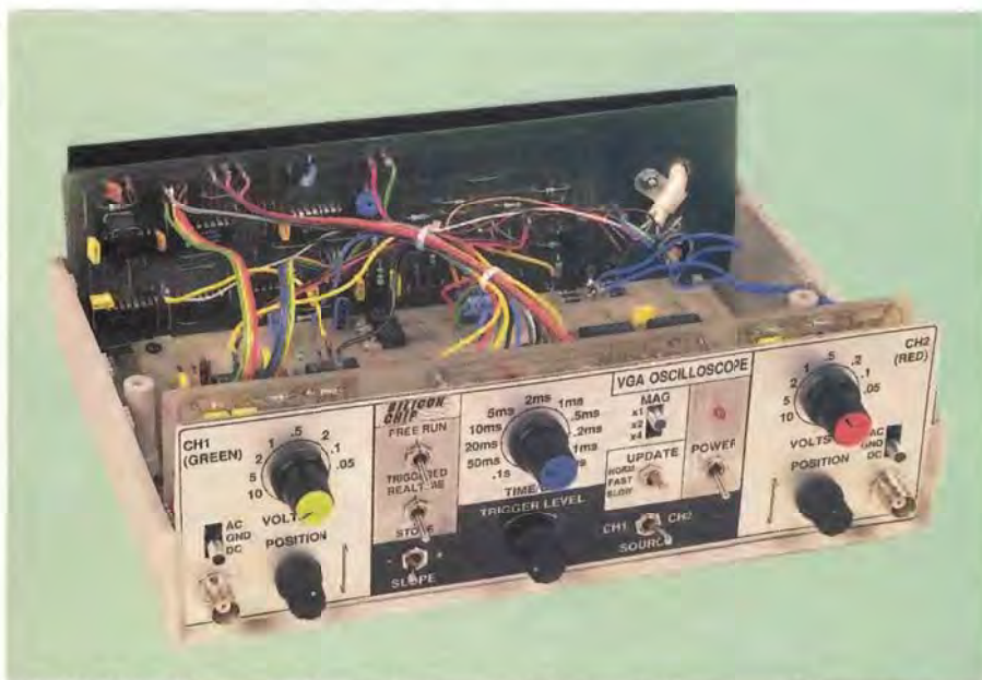
The VGA Oscilloscope adaptor has most of the controls you would expect to find on a conventional oscilloscope. Vertical input sensitivity ranges from 50mV/div to 10V/div.
