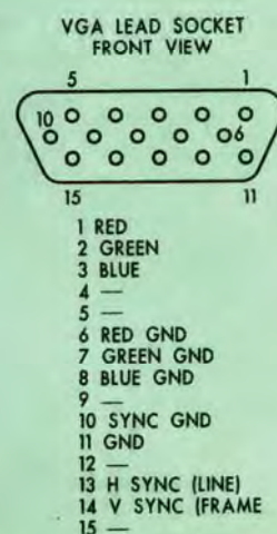
Fig.6 (above): the standard pin-outs for a VGA socket.
