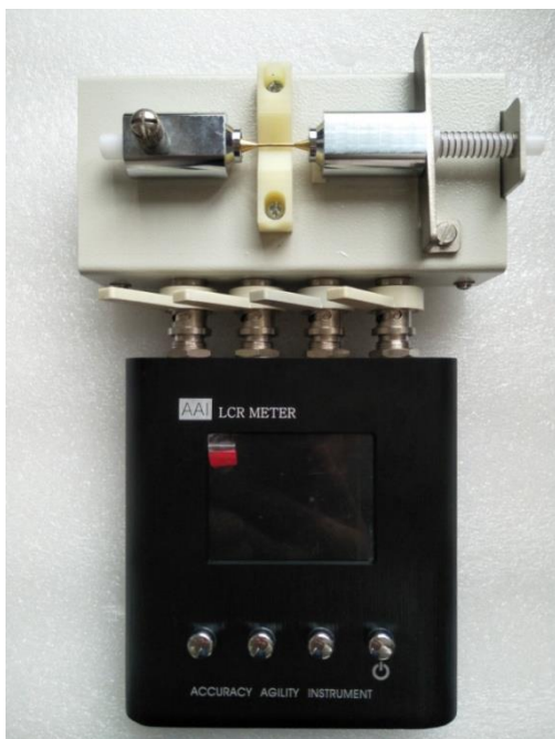
Figure 5—1 Thimble type test stand
