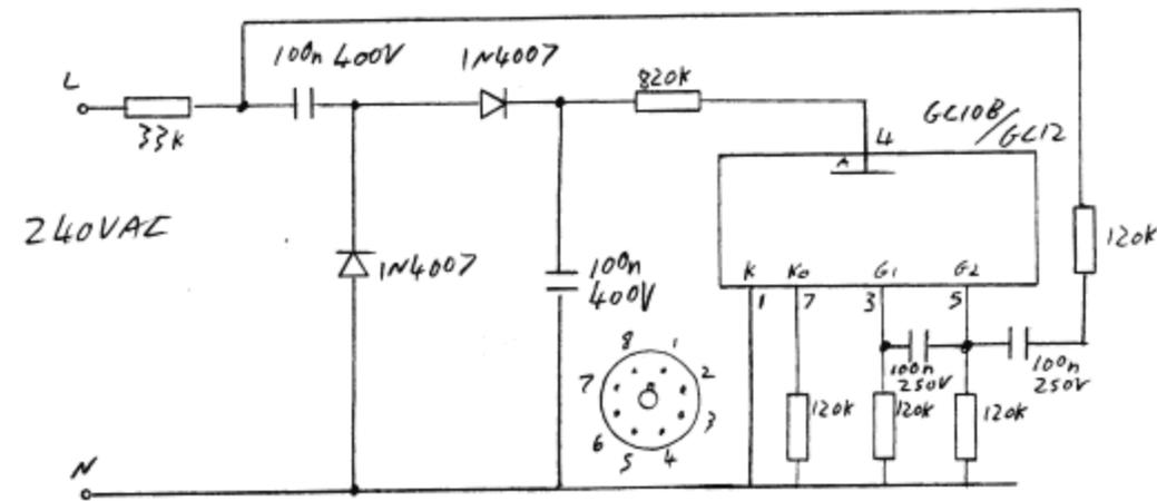
The octal base drawing is the underside view, i.e. looking at the pins. Component values are not too critical - I used what I had available. Resistors should be half-watt carbon film, or 1/4 watt metal-glaze to ensure that their voltage rating is sufficient.
