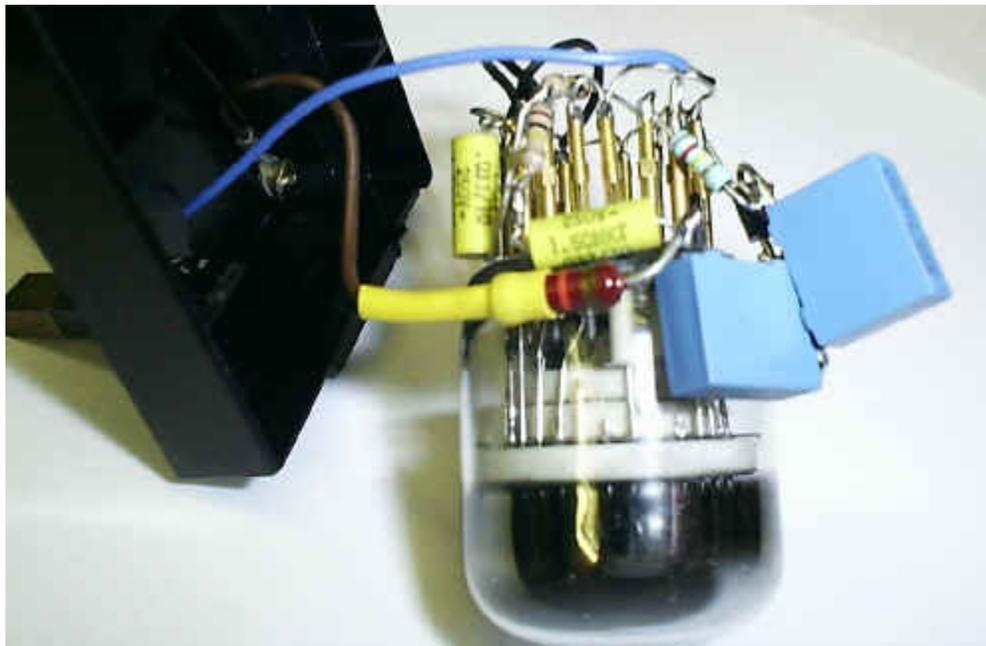
2-stage dekatron spinner from Vaughn Wright. Q1 is a high-voltage N-Channel MOSFET
