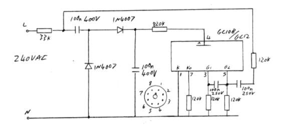
The octal base drawing is the underside view, i.e. looking at the pins. Component values are not too critical - I used what I had available. Resistors should be half-watt carbon film, or 1/4 watt metal-glaze to ensure that their voltage rating is sufficient.
