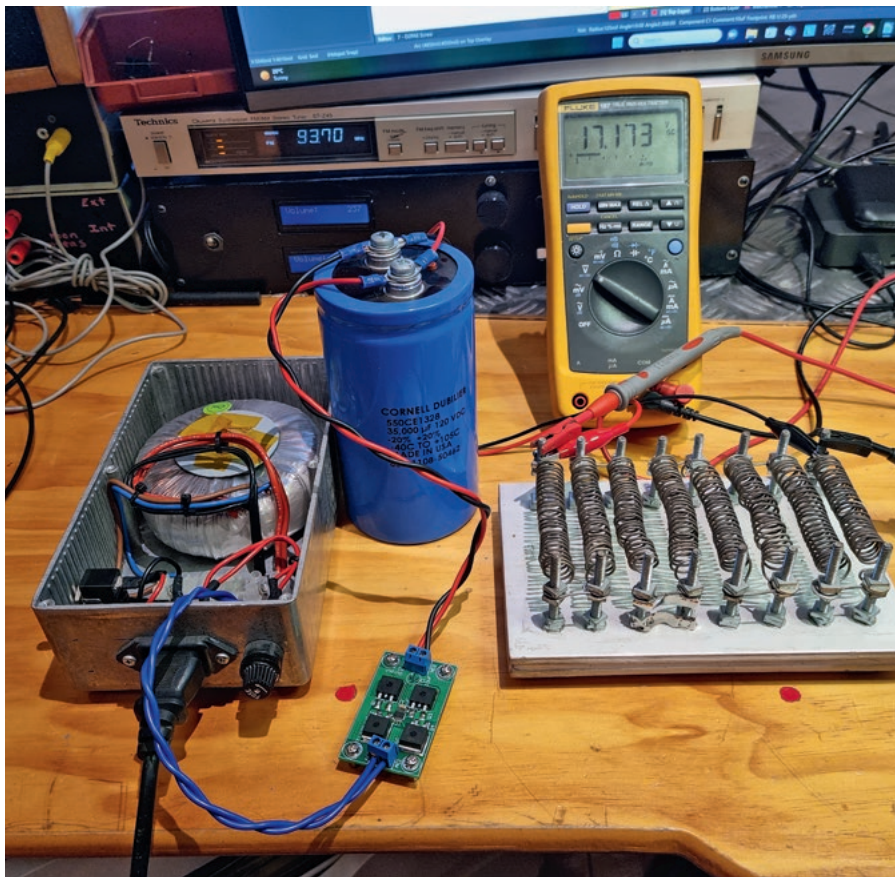
My poor wirewound nichrome dummy load reached 320°C while the Mosfets on the D2PAK standalone module only reached 67°C.
