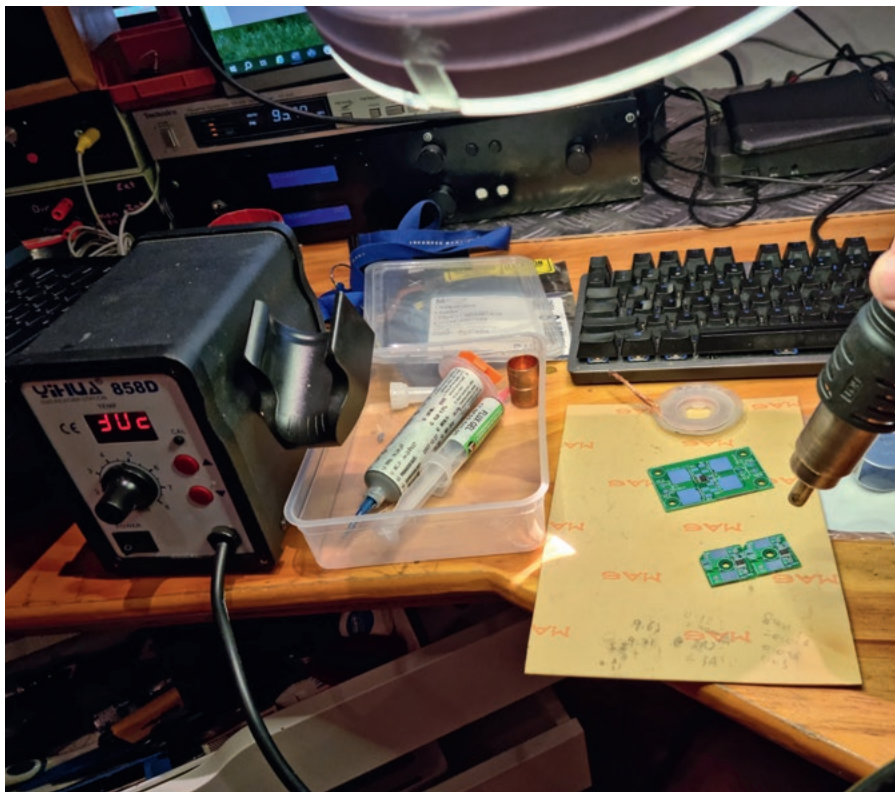
Soldering the MSOP-12 LT4320 IC using a low-cost hot air ‘rework’ station. These are invaluable for all sorts of jobs; they make it especially easy to desolder SMDs. In this case, the killer feature is the ability to heat the IC enough to solder the pad underneath.
