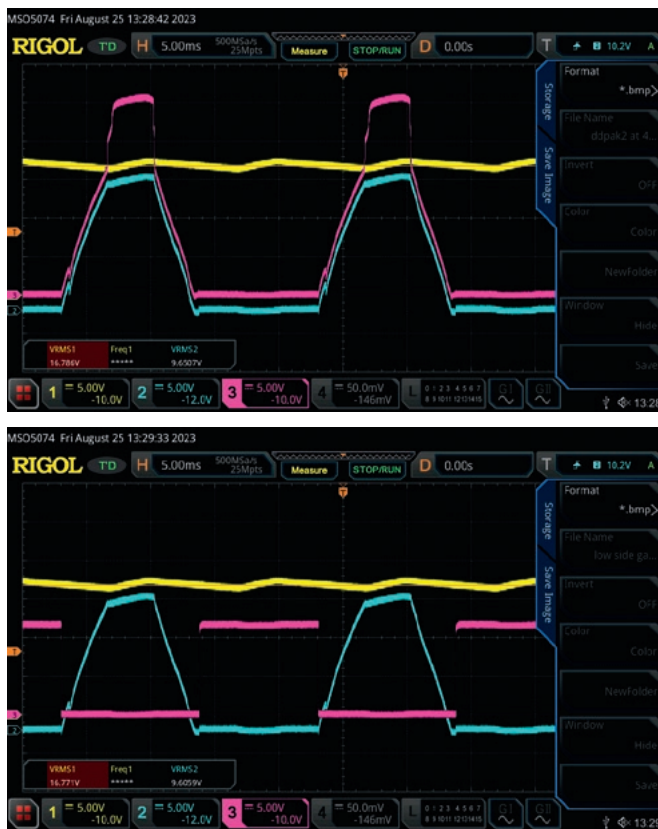
Fig.3: the cyan trace is the positive portion of the incoming AC waveform, yellow is the filtered DC output, while mauve is the positive Mosfet gate drive. The cyan AC trace is offset by -2V; otherwise, the mauve trace would obscure it much of the time.
