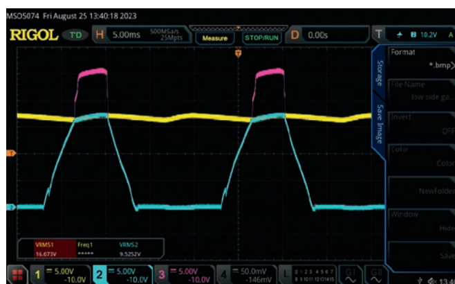
Fig.5: the same waveforms as in Fig.2 but without the -2V offset on the AC input. The IPP083N10N Mosfets on this board stabilised at 38°C in the lab. The dummy load, on the other hand, measured 130°C.
