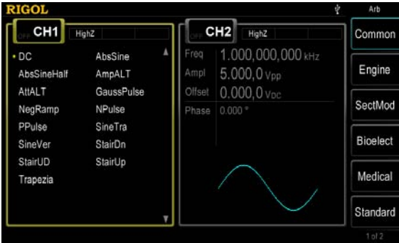
Arbitrary waveform function and built-in 150 waveforms
