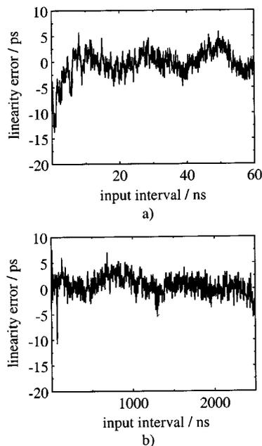
Fig. 5. Measured linearity of the TDC. (a) Input increment 65 ps. (b) Input increment 1.6 ns.
