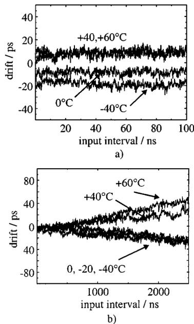
Fig. 6. Measured output error of the TDC compared to room temperature. (a) Drift due to the TDC itself. (b) Temperature dependence due to the reference oscillator.
