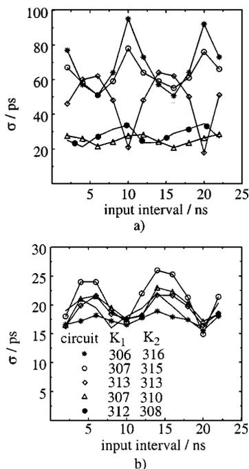
Fig. 4. Single-shot precision of TDC for five circuits. (a) Results calculated with the average stretch factor. (b) Results calculated with the real stretch factors  $K_1$  and  $K_2$  specific to the circuit.
