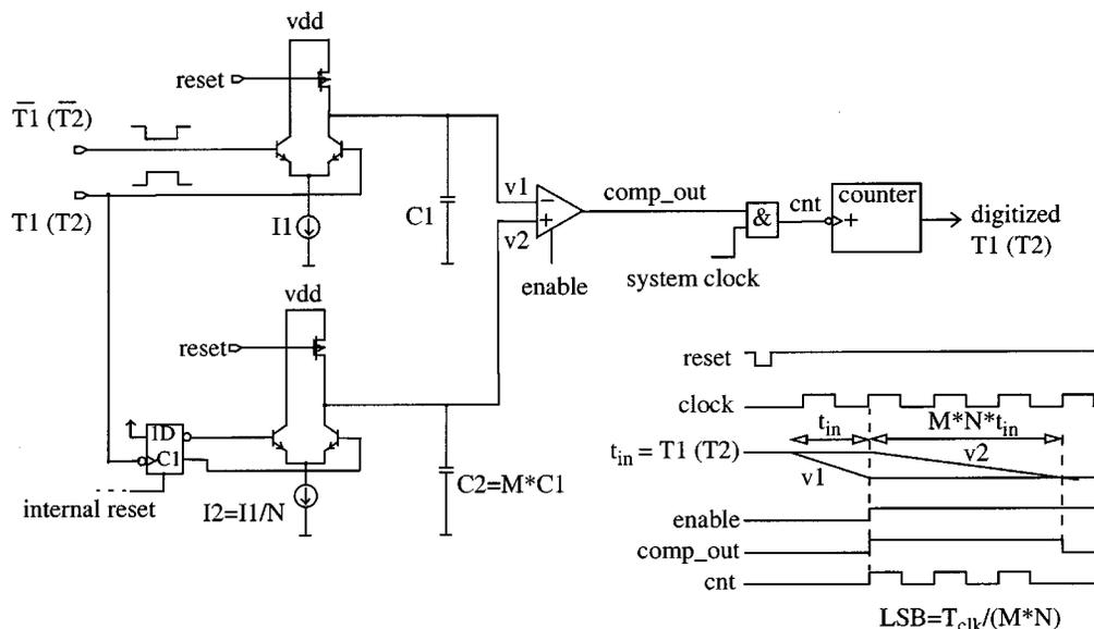
Fig. 3. Principle of the interpolator based on time-to-voltage conversion.
