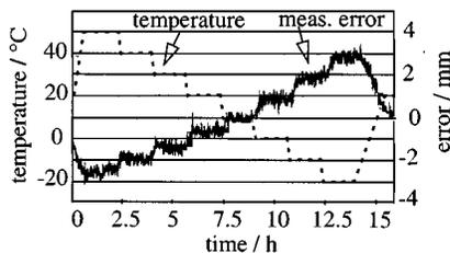
Fig. 7. Effect of the temperature on the offset of one TDC chip when a constant input interval of 50 ns (corresponding to a distance of 7.5 m) is measured.
