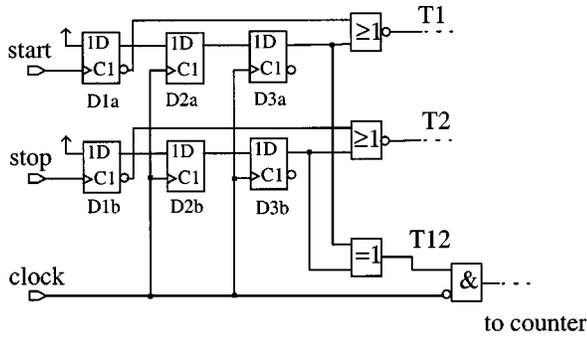
Fig. 2. Synchronization of start and stop inputs.
