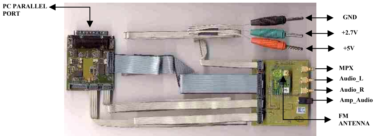
Figure 34 connection of TEA5767/68 demo board
