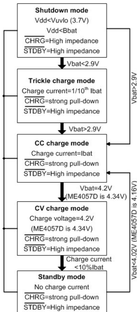
Fig.1 State diagram of a typical charge cycle
